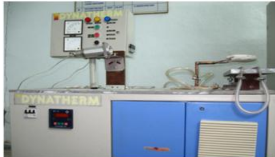
Fig 2.2.: Induction furnace used for heating the equipment.
