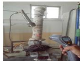
Fig 2.4: Measuring temperature by pyrometer.
